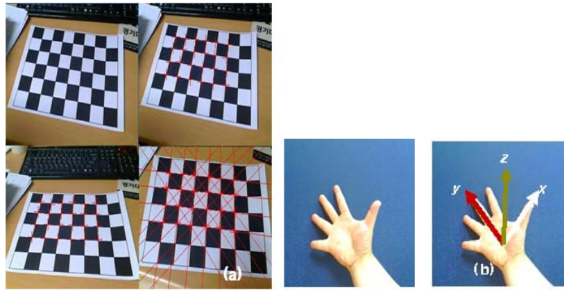
Fig. 5. (a) Grid pattern and hand posture for camera pose estimation and (b) 3D hand coordinate system
