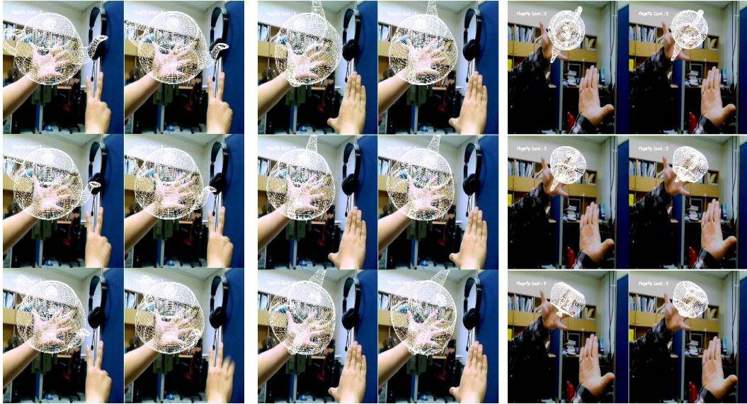
Fig. 11. Manipulation of a 3D teapot with complex background (from top left, clockwise, translation, zoom in, zoom out, rotation by z-axis, x-axis, and y-axis respectively)
