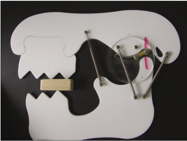
Fig. 2. Template appliance, which is located at the posterior segment of occlusal arch, reduces the pressure to the temporomandibular joint according to the 2nd principle of lever action.
