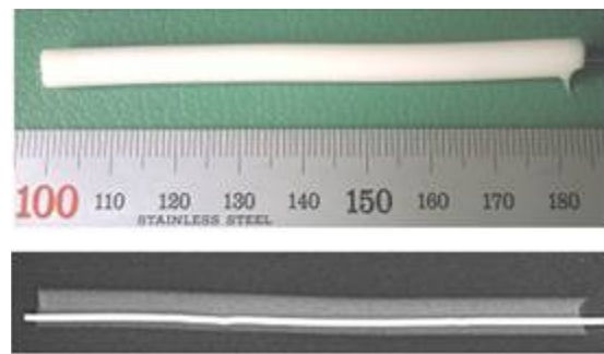
Figure 1. Tissue phantom with a steel wire (up) and its X-ray image (down).
