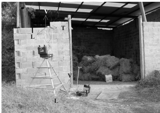
Fig. 3. Measurement of blasting vibration on ground and structure
