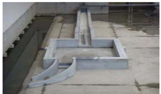
Fig. 5. Model of the discharge channel.
