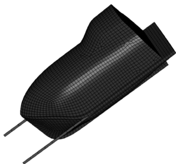
Fig. 6 Configuration of F.E. mesh of lifeboat and skid models
