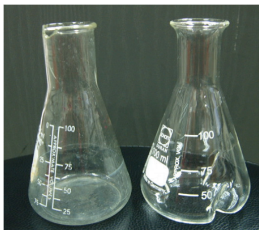
Fig. 2. Picture of different flasks. Left: normal erlenmeyer flask, right: baffled erlenmeyer flask.
