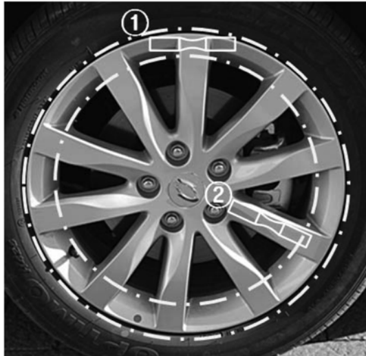
Fig. 1. Photograph of a vehicle wheel indicates specimen sections for tensile and fatigue test.
