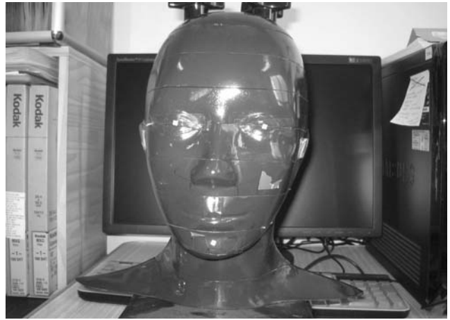
Fig. 1. Female adult ART head and neck phantom was used for the dosimeter location.
