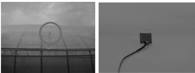
Fig. 4 Location of heat flow sensor on greenhouse surface
