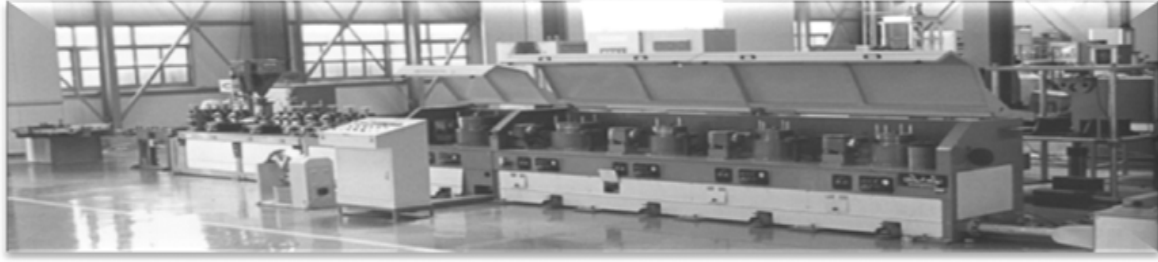
Fig. 7 Pilot line for the production of metal cored welding wire
