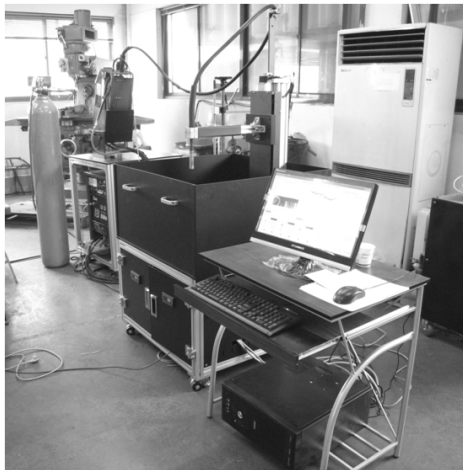
Fig. 8 GMA welding station
