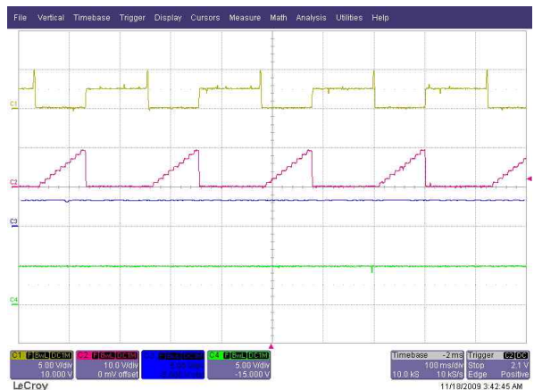
MODE[1/2.5V], speed_ss_flag[1/1V], fault_index[1/1V], fault_flag[1/5V] (b) 고정자 권선 1/24 단락 (FTR=4.17%)
