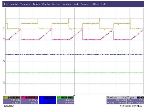
MODE[1/2.5V], speed_ss_flag[1/1V], fault_index[1/1V], fault_flag[1/5V] (a) 고정자 권선 1/36 단락 (FTR=2.78%)
