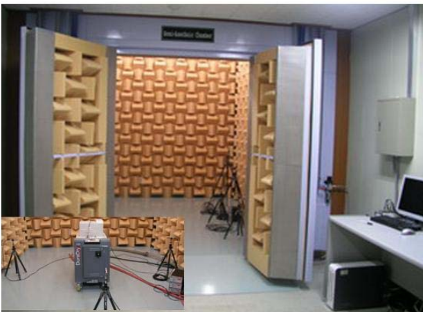
Figure 5. Performance evaluation systems for dry vacuum pump.
