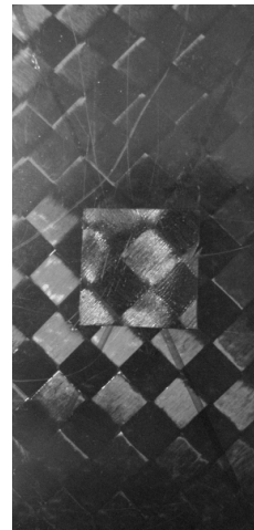
Fig. 9. Application of external patch
