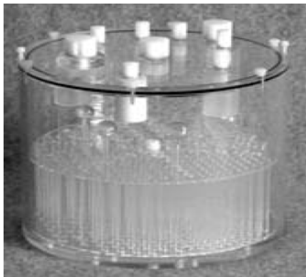
Fig. 2. Flangeless esser PET phantom from Data Spectrum Corporation
