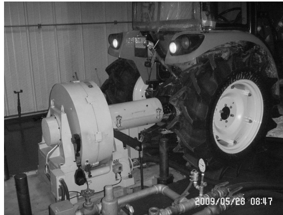
Fig. 1 Tractor PTO power test.
