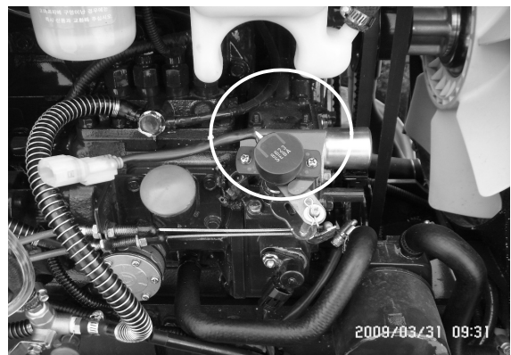
Fig. 2 Potentiometer for measuring throttle opening angle.
