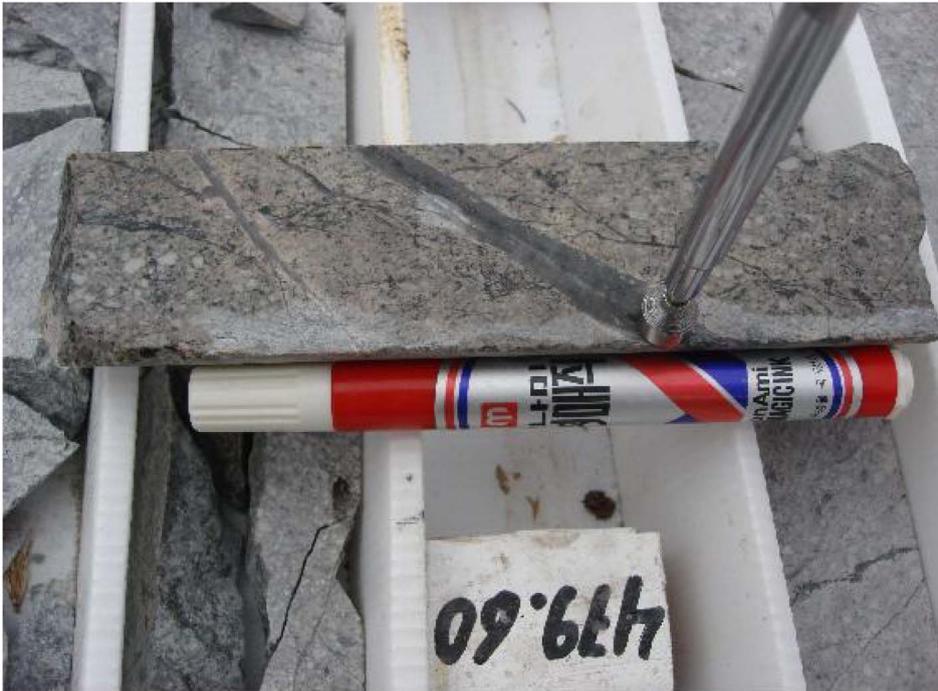
**Fig. 6.** Photographs showing magnetite-bearing M type vein from the Ccalla porphyry.
