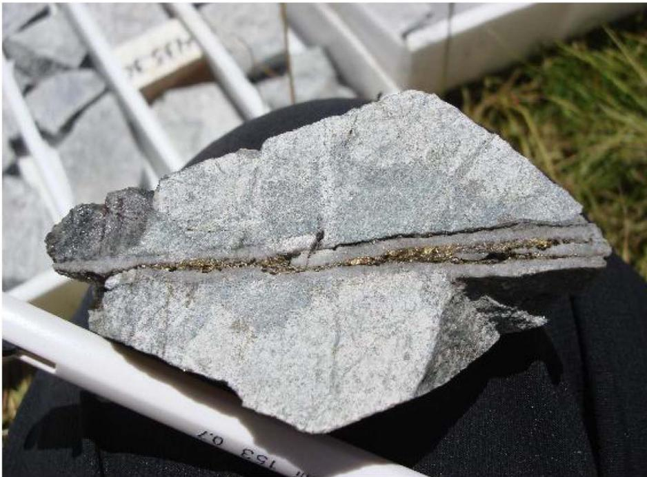
**Fig. 7.** Photographs showing the B type vein from the Ccalla porphyry. The quartz-chalcopyrite vein is characterized by sulfides along center lines with encompassing quartz.
