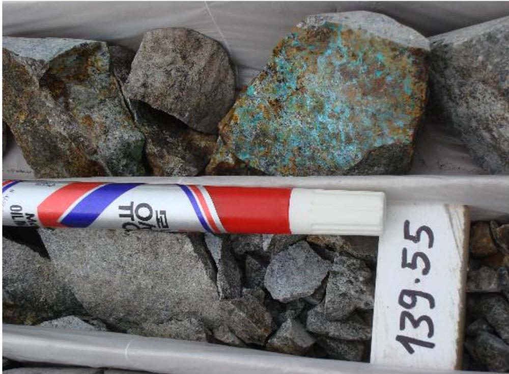
Fig. 4. Copper oxide zone observed in drill core (139.55 m).
