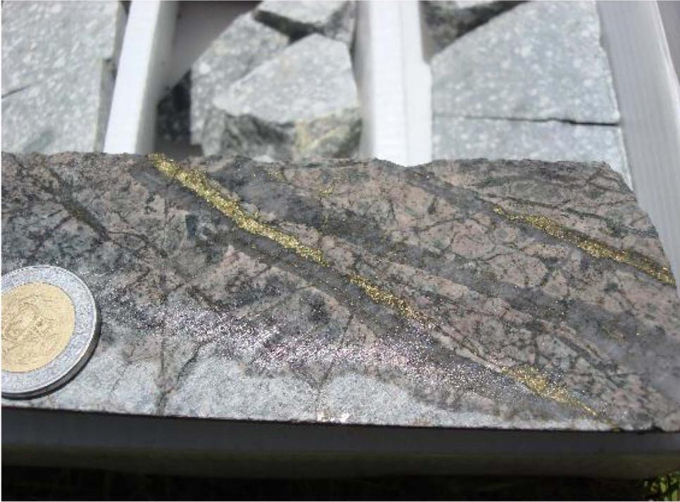
Fig. 5. Photographs showing the quartz-chalcopyrite veins infilling the fractures from the Ccalla porphyry.
