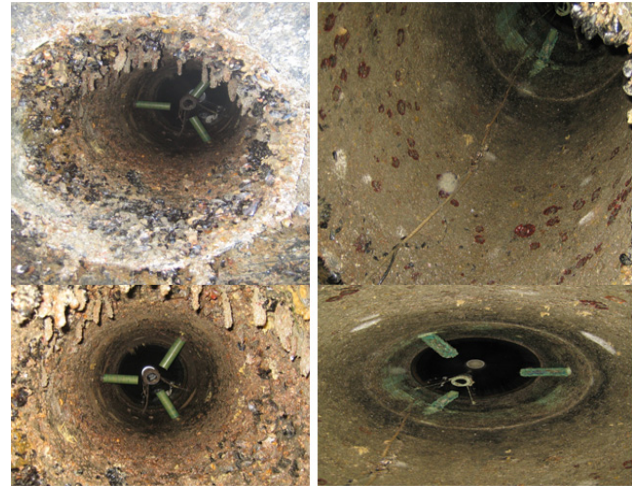
Fig. 8 Photograph of Operation results of AFS (Left : inactive AFS , Right : active AFS)
