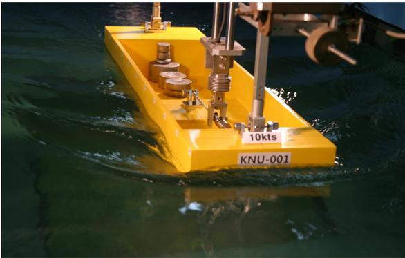
Fig. 9 Wave patterns for KNU-001 (full load condition, V=10 knots)
