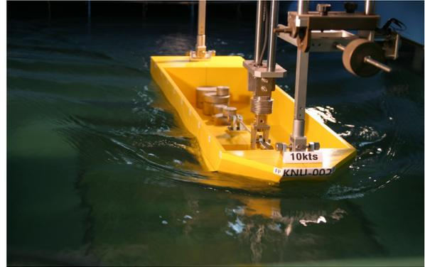
Fig. 12 Wave patterns for KNU-002 (full load condition, V=10 knots)
