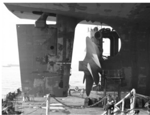
Fig. 1 Typical profile of the rudder erosion
