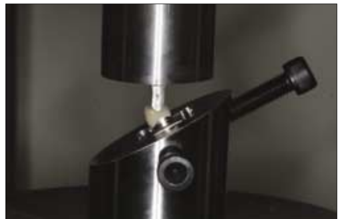
Fig. 5. Fracture strength test of zirconia ceramic crown using the universal testing machine.
