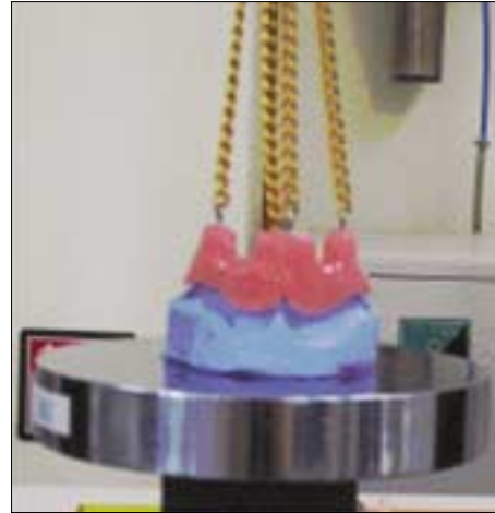
Fig. 3. The vertically directed dislodging force applied to the resin base sample.
