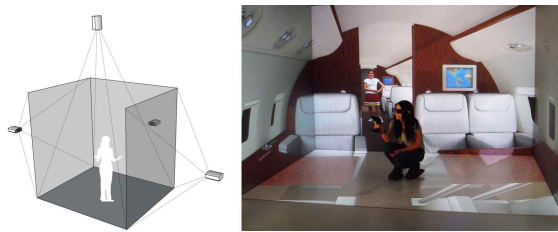
Figure 1. Four-wall CAVE system configuration(left) and an application example(right)
