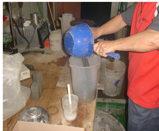
Fig. 1 Preparation of cement milk
