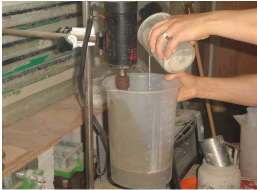
Fig. 3 Preparation of thixotropic grout mortar
