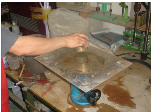
(a) Initial mortar flow before impaction
