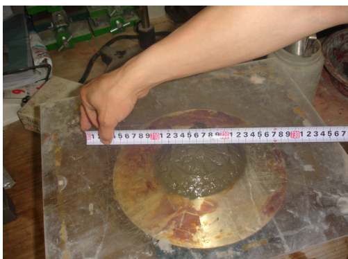
(b) Mortar flow after impaction 15 times
