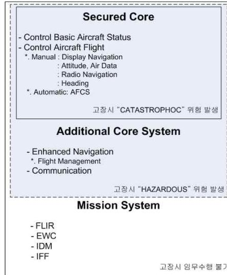
Fig. 2. Safety Requirements for Subsystems
