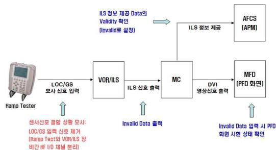
**Fig. 9. Sensor safety test using LOC/GS simulator**
