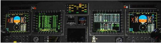
Fig. 1. Glass Cockpit Display of KUH (Surion)
