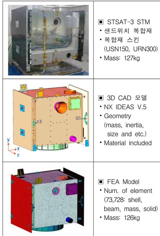
**Fig. 4. The STSAT-3 full model of real, cad and fea**
