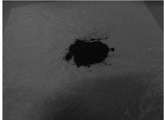
Fig. 2. Photograph of the vanadium pentoxide sample grinded.
