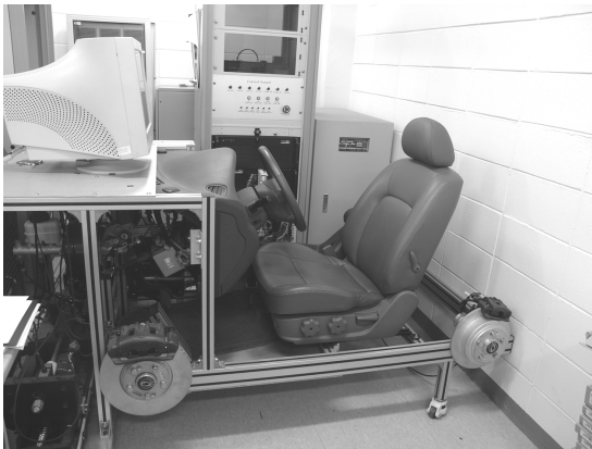
Fig. 4 HILS system for SMC-ABS test
