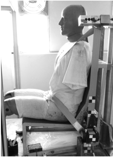
Fig. 2 Experimental set-up of the pretensioning system
