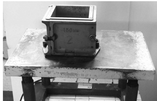
Fig. 2 Vibro-compaction by the vibrating table.
