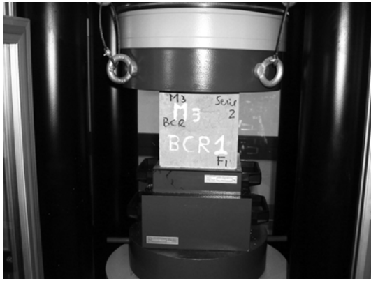
Fig. 4 Compression of the RCC specimen according to one of the three various facets.
