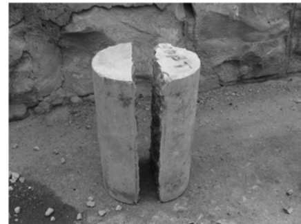
(b) Failure pattern of samples after tensile strength test
