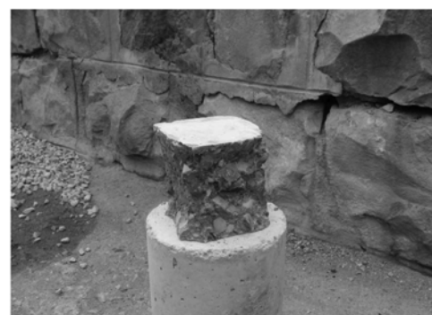
(b) Failure pattern of samples after compressive strength test
