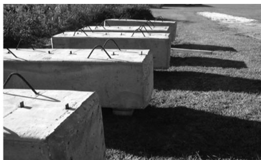
Fig. 6 Piles with embedded metal plates.
