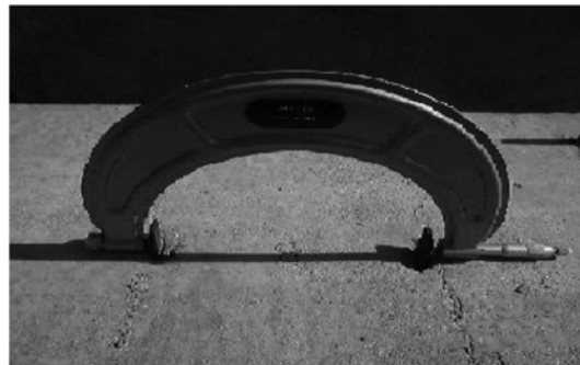
Fig. 7 Micrometer measurement of embedded plate distance.
