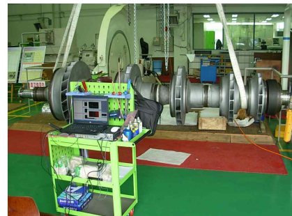
Fig. 4 Modal testing of ATC rotor
