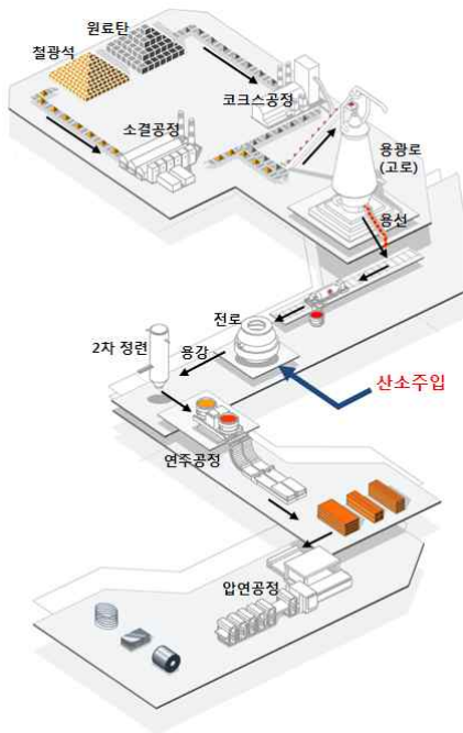
Fig. 1 Manufacturing process of steel products
