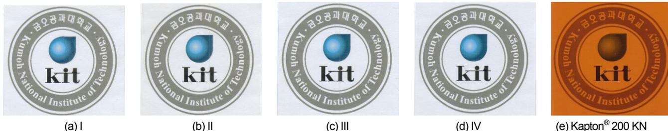
Figure 6. Photographs of PI films with various diamines: (a) I; (b) II; (c) III; (d) IV. Kapton® 200 KN was shown in (e) as a reference.
