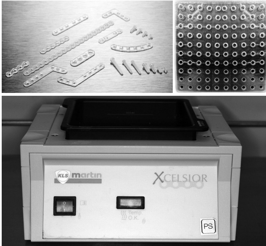
Fig. 1. (Above, left) Shapes of commercially available absorbable plates, screws and (Above, right) mesh (photograph supplied by manufacturer). (Below) Water bath system used for heating the absorbable mesh to a malleable form.
