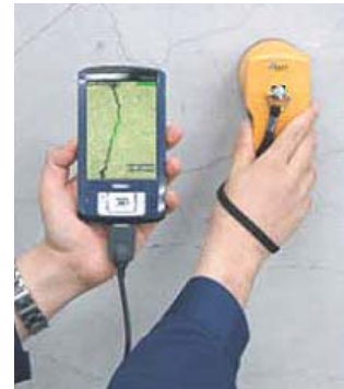
휴대용 균열측정기(CRACK K VIEWER)
