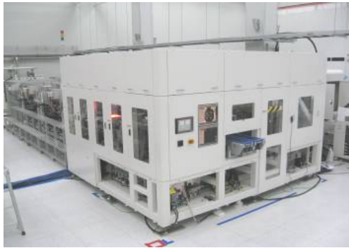
Figure 1. Dry etching chamber system for texturing using plasma.
