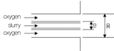
(b) simplified burner design
