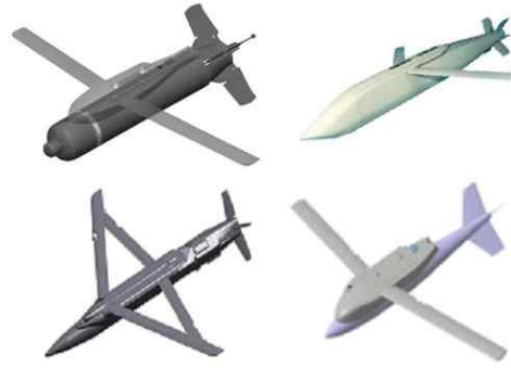
Fig. 1. Air to ground flying bombs with high aspect ratio wing (non-propellent)
