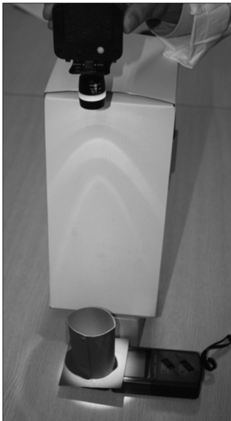
Fig. 7. Measurement of intensity of illumination by photometer (Distance 40cm ; photometer- light source).
