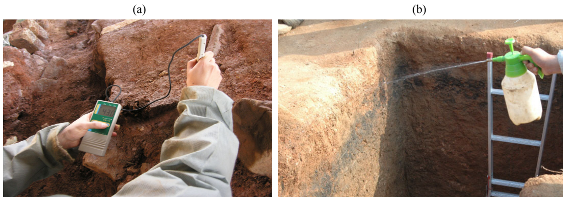
Figure 1. Preliminary investigation method. (a) Measurement of containing water in soil layer. (b) Add moisture into dry layer.
