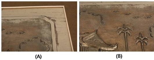
Figure 9. Contamination (A) and discoloration (B) on the surface.
