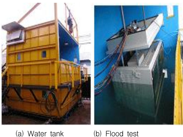
Fig. 6. Water tank and flood test
