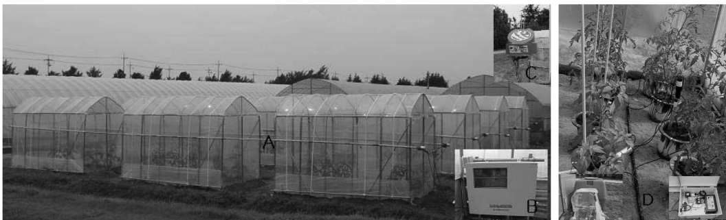
Fig. 1. View of experimental small greenhouses (A), a side-window controller (B), a rain sensor (C), and tomato and pepper potted-plants grown by automatic irrigation system based on soil moisture contents (D).
