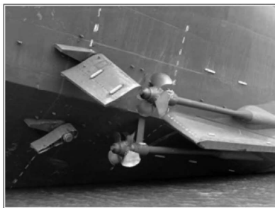
(b) damaged rudders and propellers
