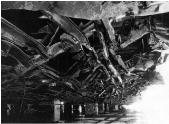
Fig. 9 Damage to the Sea Empress after multiple shallow grounding events
