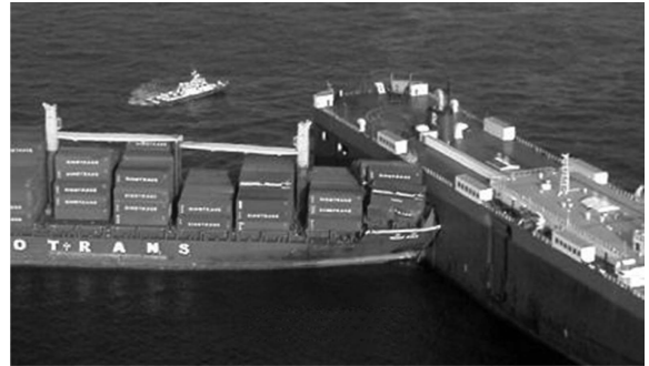
Fig. 4 Collision accident of container ship and car carrier
