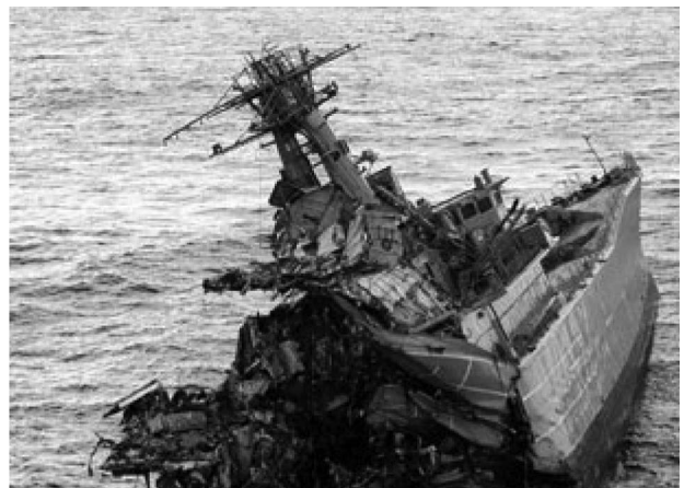
Fig. 12 Damaged Australian destroyer Torrance due to underwater explosion
