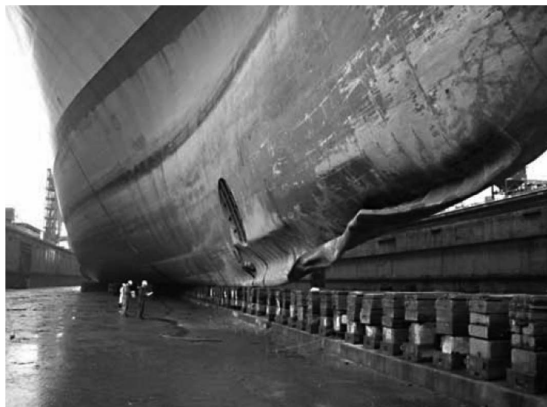
Fig. 10 Grounding damage of Maersk Kendal showing a longitudinal cutting of bottom shell
