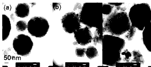
Fig. 11 TEM image for fresh and aged catalysts [(a) fresh (b) 700°C 36 h aging (c) 800°C 24 h aging (×100K)]
