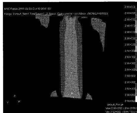
Fig. 12 von Mises stress distribution of aluminum liner at autofrettage pressure for path dependant crack model.
