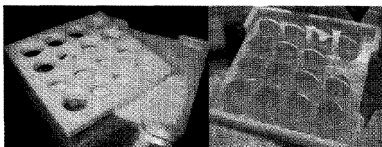
Fig. 3 Photograph of the mold for agarose scaffold
