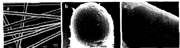
Fig. 9. a) carbon fibers with the diameter of 7.1 \mu\text{m} , b) cross-sectional image of the fiber showing the diffusion-reacted MgB 2 shell layer, and c) fractured MgB 2 layer showing the pore-free dense microstructure.
