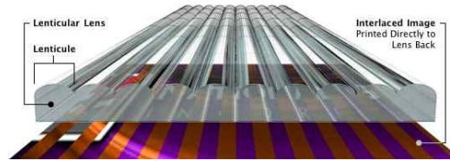
<Fig. 9> A schematic representation of Interlaced Image.
