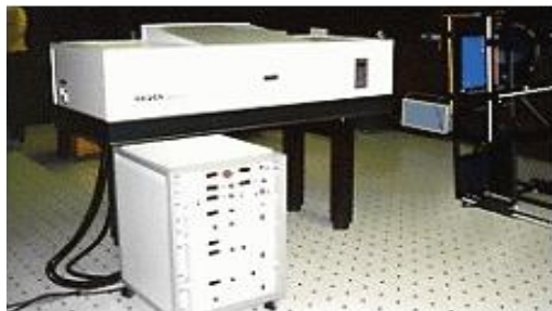
<Fig. 4> Pulsed holography camera GP-2J in pulsed hologram studio in Korea 22) .
